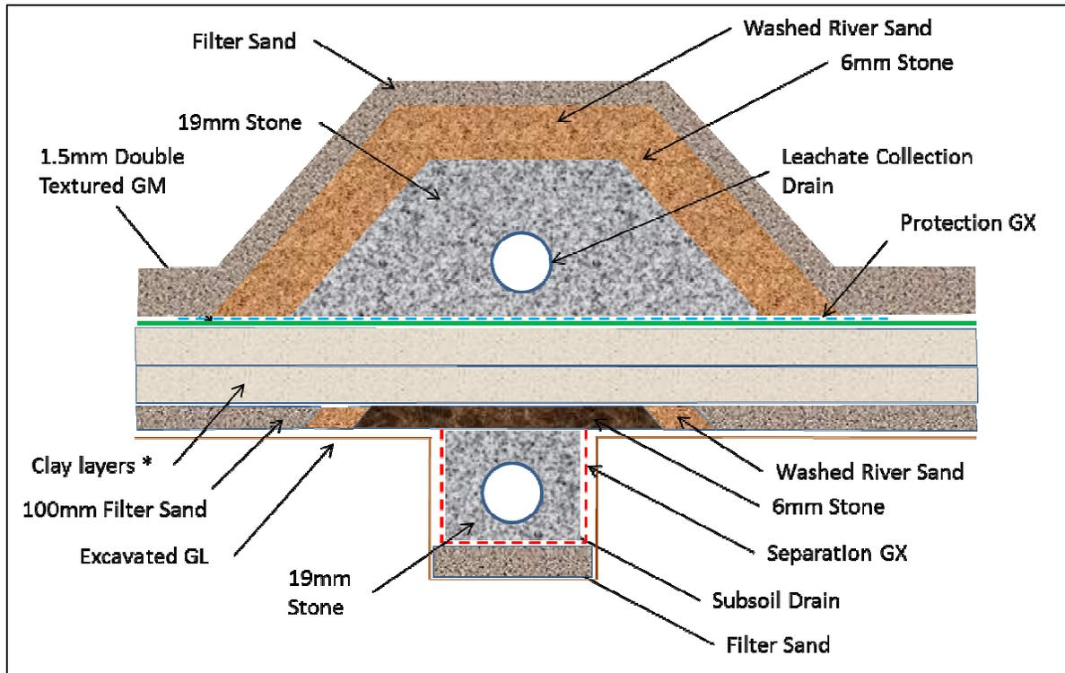
**Figure 1:** Proposed Liner System for the Eskom Kusile Power Station Project 60 Year Ash Dump
