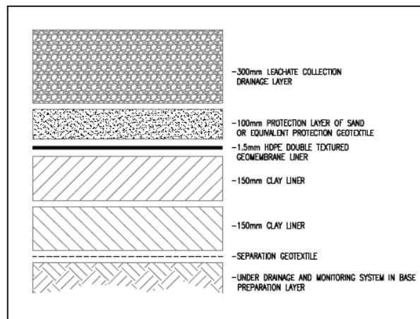
**Figure 4: Class C Liner Specification**
