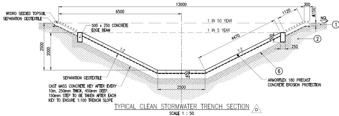
**Figure 9: Detail for clean storm water canals**
