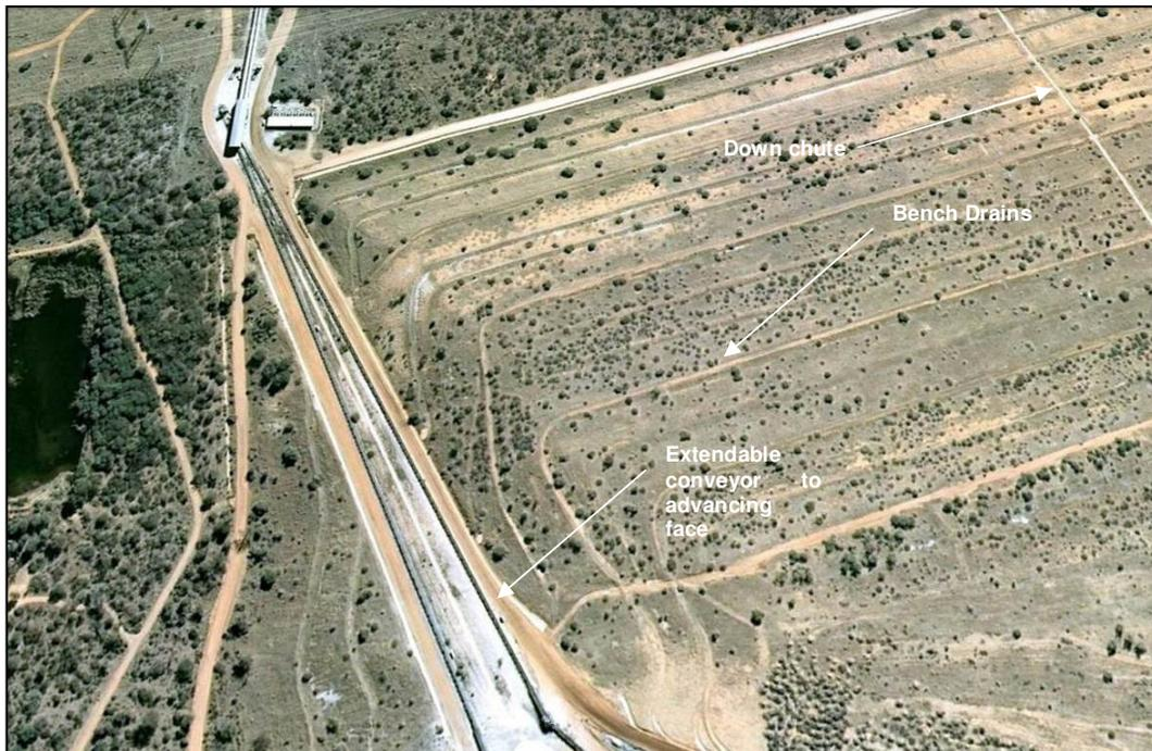
Figure 11: Rehabilitation of Matimba's ash facility
