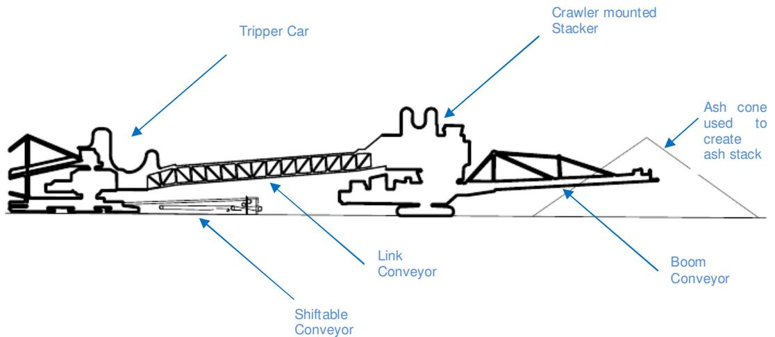
**Figure 13 : Stacker setup**
