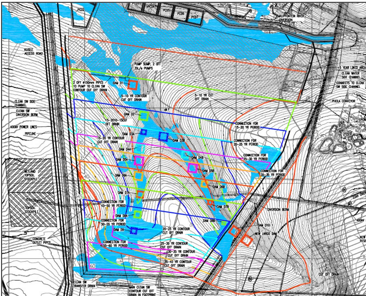
**Figure 6: Layout of Clean Storm Water Dams and Pollution Control Dams**
