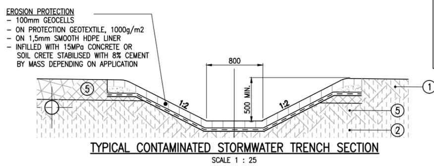
**TYPICAL CONTAMINATED STORMWATER TRENCH SECTION**
