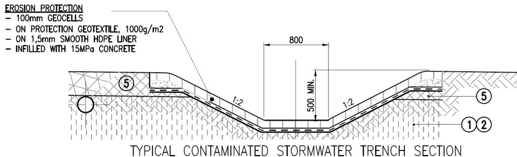
**Figure 8: Detail for contaminated storm water canals**
