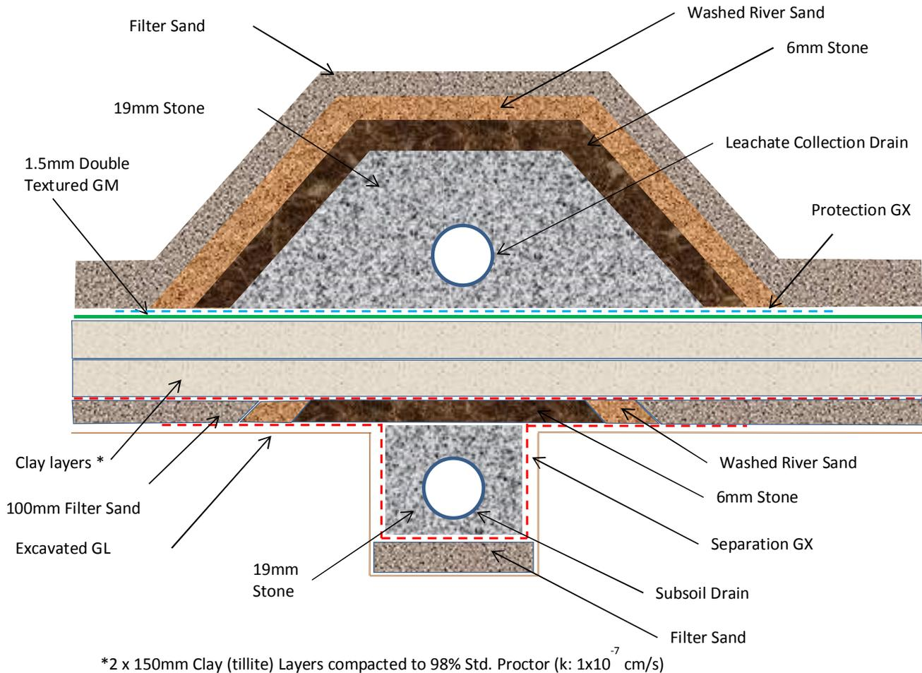
**Figure 5: Lining system applied to site conditions showing leachate and sub-soil conditions**
