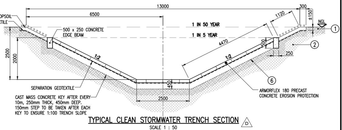
**TYPICAL CLEAN STORMWATER TRENCH SECTION**
