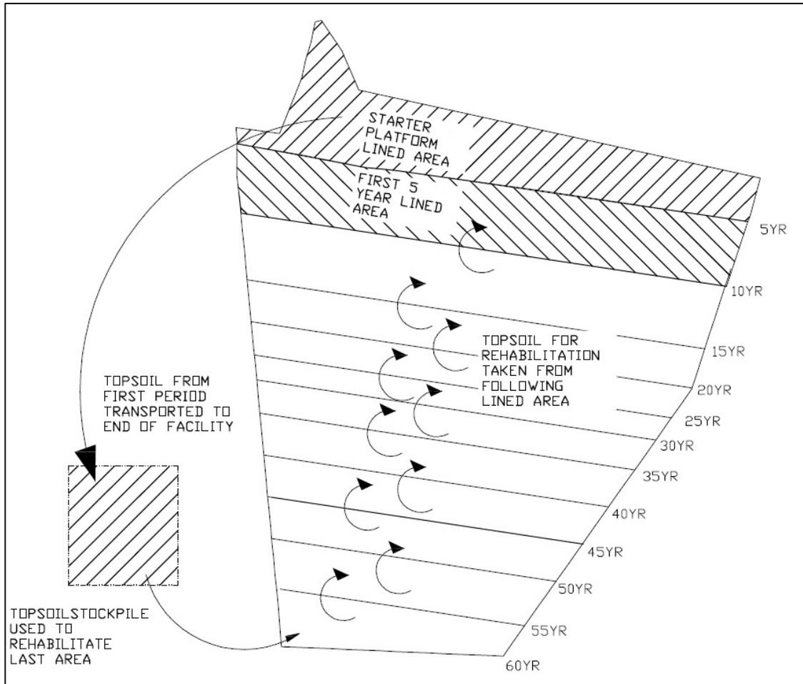
**Figure 18: Method of progressive topsoil management**
